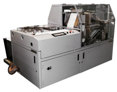
The Tripla TC 7900 can process large paper format, up to 760 mm continuous paper modules printed in 3-up mode
