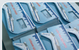
Form- and die cut in one step
