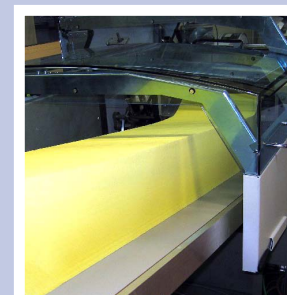
Open design allows for web inspection at any time
